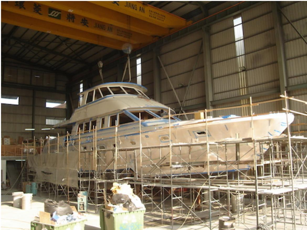
The hull and deck are faired for gel coating and painting, and the frameless windows will be installed throughout the semi-custom yacht to maintain the clean profile. Once the fairing is complete, the yacht will be ready to paint.
