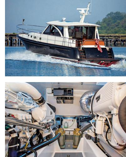
LOA: 45'10" BEAM: 14'6" DRAFT: 4'0" (props) DISPL: 35,000 lb. (half load) FUEL: 450 gal. WATER: 120 gal. DEADRISE: 20 degrees ENGINES (tested): 2 x 593 hp Cummins QSC8.3 600 diesels w/ ZF pod drives ENGINES (std.): 2 x 450 hp Caterpillar C7 ACERT diesels BASE PRICE: \$1,350,00
